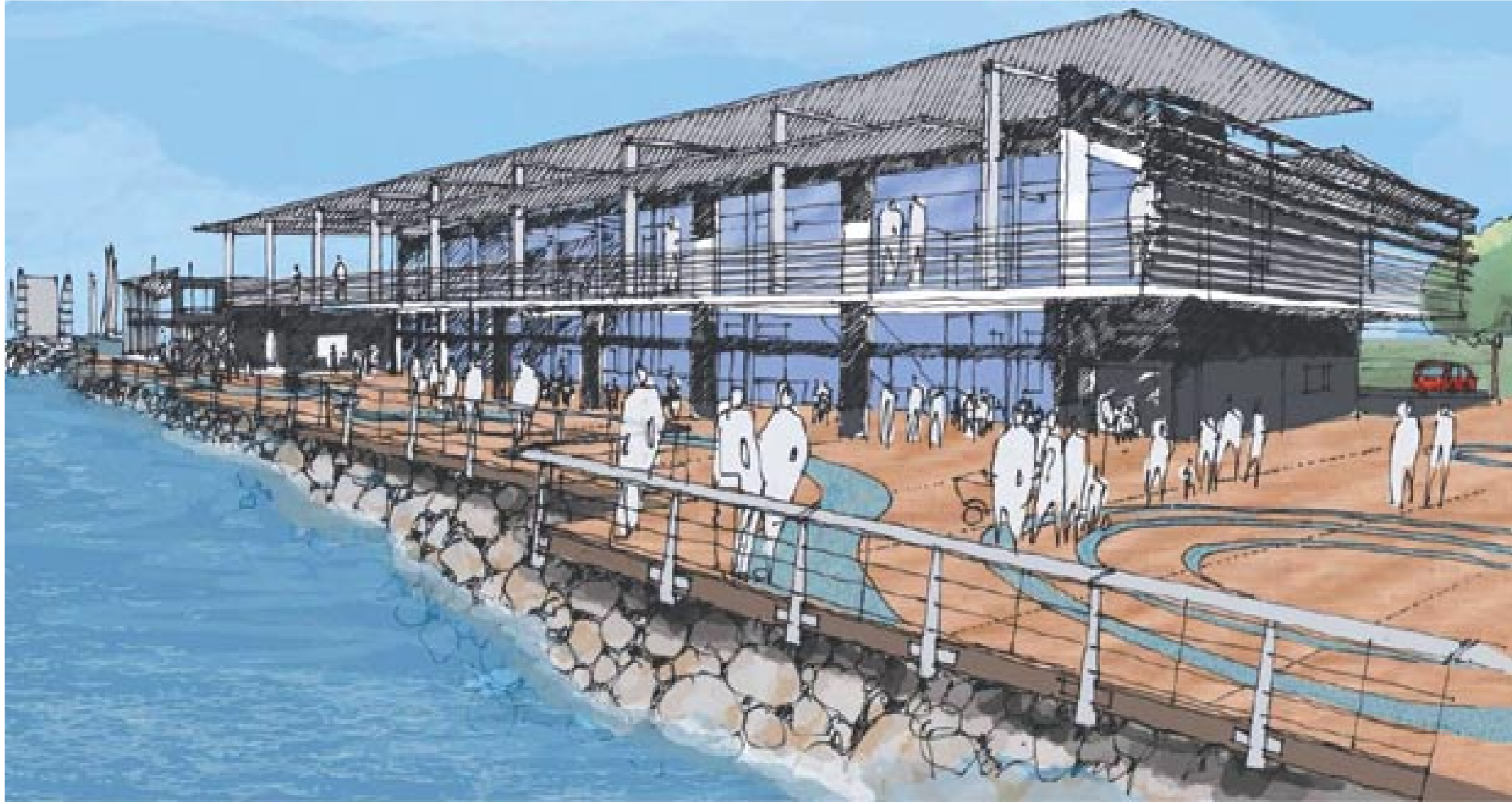
Verandahs and eaves will provide shade in summer but allow light and warmth into buildings in winter
